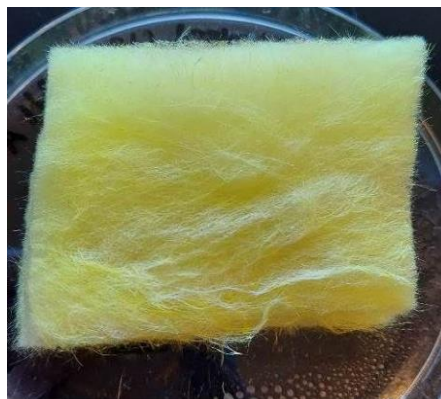
Figure 2. Glass Wool Blanket UET GB 0221 Post-Incubation Close-Up
